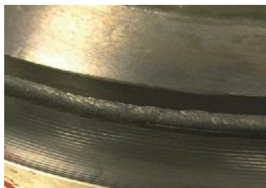
Welded seam OK
