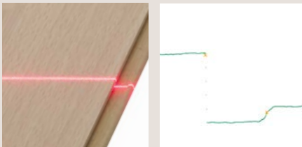
Profile inspection of parquet board edges
