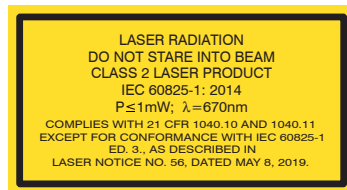
Fig. 1 Laser labels on the sensor cable
