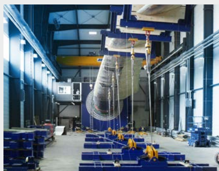
Measuring the deformation of rotor blades for wind turbines
