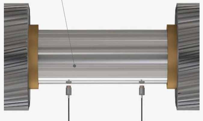
Run-out monitoring of gear shafts
