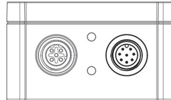
Fig. 31 Supply and analog output controller, 8-pin male connector
