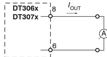
Fig. 34 Wiring for current output
