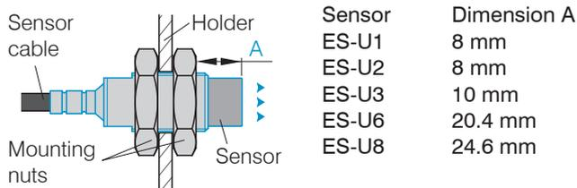
Fig. 5 Unshielded sensor with thread in standard mounting
