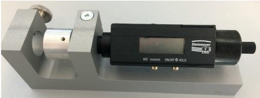
A precision micrometer calibration unit. It consists of a black cylindrical sensor mounted on a silver metal base. The sensor has a digital display and control buttons. The base has a threaded hole for mounting. | <p>Micrometer calibration unit<br/>Setting range: 0-2.5 mm,<br/>with digital position reading<br/>and adjustable zero,<br/>for sensors type ES04-ES2 resp. type U05-S2</p> |
