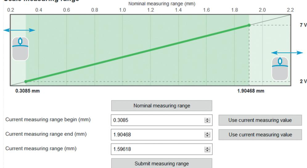
Fig. 38 Scaling the measuring range using the pointer
