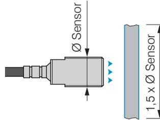
*Fig. 28 Minimum target size for shielded sensors*
