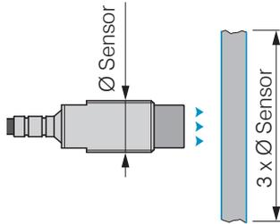
*Fig. 27 Minimum target size for unshielded sensors*
