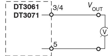
Fig. 35 Circuit of temperature measurement
