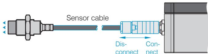
To release the plug-in connection, hold the plug-in connector on the grooved grips (outer sleeves) and pull apart in a straight line.
