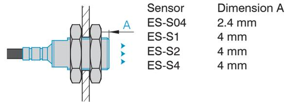
Fig. 6 Shielded sensor with thread in standard mounting
