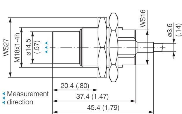
Fig. 21 Dimensional drawing sensors ES-U6-C-CAx/mB0
