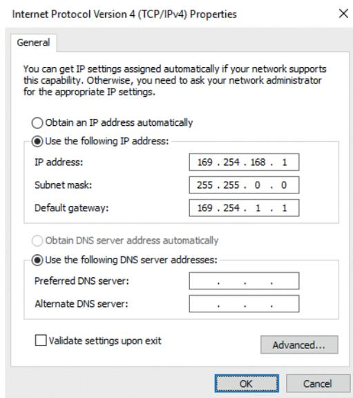
The IP address of the controller is factory-set to 169.254.168.150.
