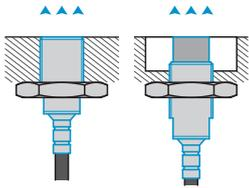
Flush mounting does not correspond to factory calibration. Micro-Epsilon recommends to carry out at least a 3-point field linearization.
