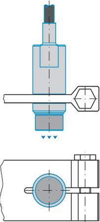
This type of sensor installation ensures the highest level of reliability because the sensor's cylindrical cover is clamped over a relatively large area. It is imperative in complex installation environments such as machines and production plants.
