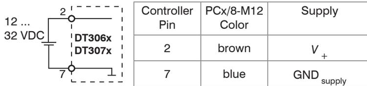
Use the supply voltage for measurement instruments only and not for drive units or similar sources of pulse interference at the same time. Micro-Epsilon recommends using an optional available power supply unit PS2020 for the controller.
