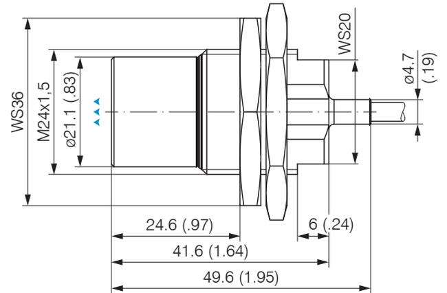
Fig. 22 Dimensional drawing sensors ES-U8-C-CAx/mB0
