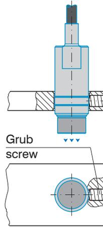
This simple type of fixture is only recommended for installation locations that are free of impact and vibration. The grub screw must be made of plastic so that it cannot damage or deform the sensor housing.
