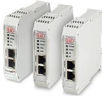
Interface module for connection to EtherCAT, PROFINET or EtherNet/IP of a Micro-Epsilon sensor with RS485 or RS422 interface; DIN rail housing, incl. device description file for software integration in the PLC
