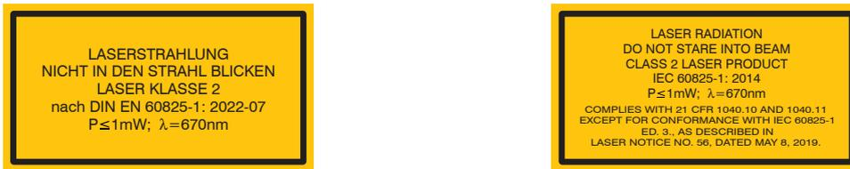
Fig. 2.1: Laser warning signs on the sensor cable
