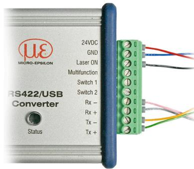
Symmetric differential signals acc. to EIA-422, not electrically isolated from supply voltage. Use a shielded cable with twisted wires.
