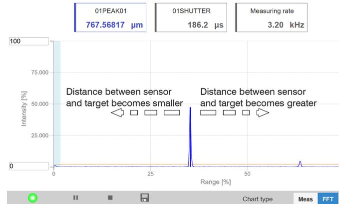
Using the FFT signal for sensor positioning
