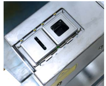
Pneumatic mechanism protects optical system from dirt
