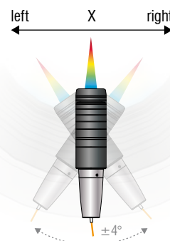
❸ Max. tilt angle in X \pm 4^\circ
