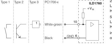
24 V loaic (HTL): Low level  $\leq$  3 V: High level  $\geq$  8 V (max 30 V) 5 V logic (TTL): Low level  $\leq 0.8$  V: High level  $\geq 2 V$ internal pull-up resistor, an
