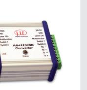
Symmetric differential signals acc. to EIA-422, not electrically isolated from supply voltage. Use a shielded cable with twisted cores e.g. PC1700-x.
