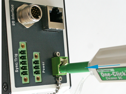
Fig. 128 One-Click™ Cleaner for cleaning E2000 optical fiber transitions
