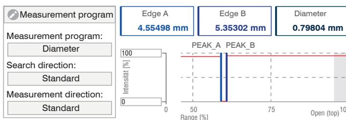
Measuring a thin, fast-moving object (e.g. wire). Signal and video averaging are disabled. The measurement provides the current measurement value at all times and is therefore insensitive to vibrations
