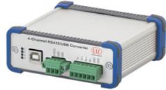
4-channel converter from RS422 to USB, suitable for cable PC/SC2700-3/IF2008; including driver, connections: 2 x sub-D, 1 x terminal block
