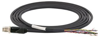
Cable for power supply, RS422 and synchronization; one side 12-pin socket M12, other side open ends; cable length x = 3 m, 5 m, 10 m, 20 m <sup>[11]</sup>
