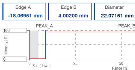
Measures the gap between two objects. The width of the gap and the angular deviations of the gap edges (AT and BT) are output. Application in rolling systems such as calender rolls.
