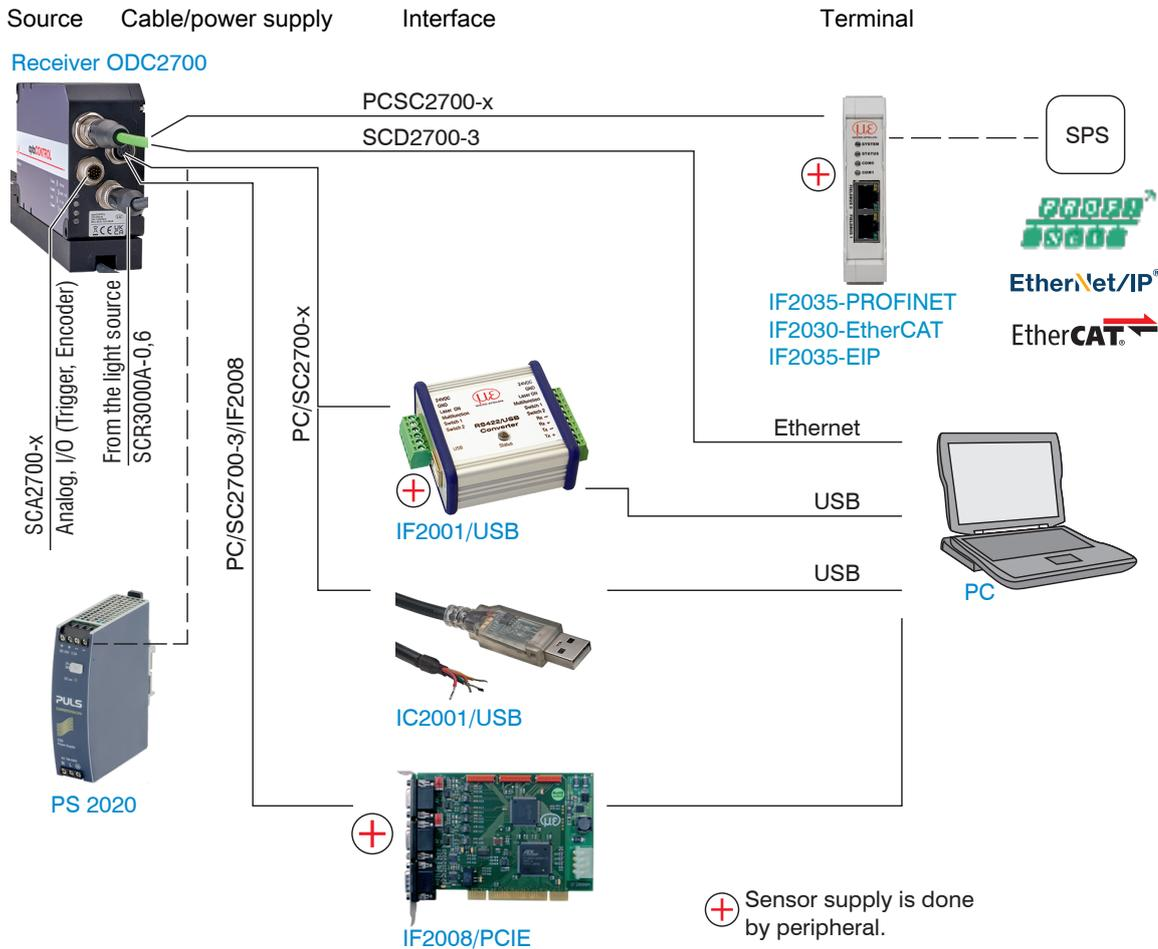
Fig. 4.2: Connection examples with the optoCONTROL 2700
