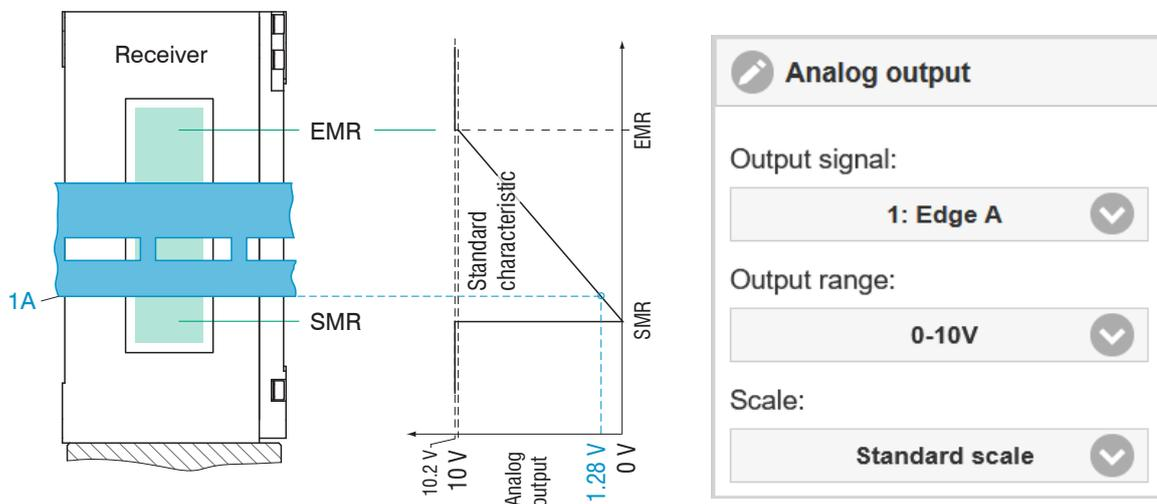
Fig. 6.23: Scaling of Analog Signal 0 ... 10 V, Example of Edge Tracing, Search and Measurement Directions: Standard
