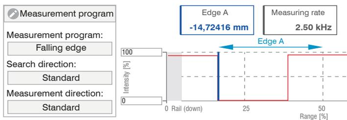
Sets the controlling and measurement of strip edges, such as paper, glass, sheet metal or film. The signal quality should be adapted to the material (paper webs - high averaging, sheet metal webs - median, film - low averaging).
