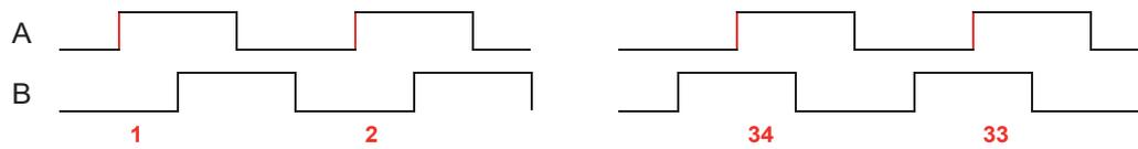
Fig. 6.1: Encoder Signal Pulse Image, Single Resolution, Add Up (Left), Decrease (Right)
