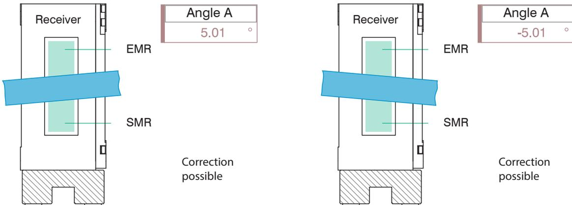
Fig. 6.8: Measurement Chart for Targets Titled Counterclockwise (Left) and Clockwise (Right)
