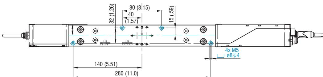
Fig. 4.3: Dimensional Drawing of Mounting Rail, Standard Mounting Method
