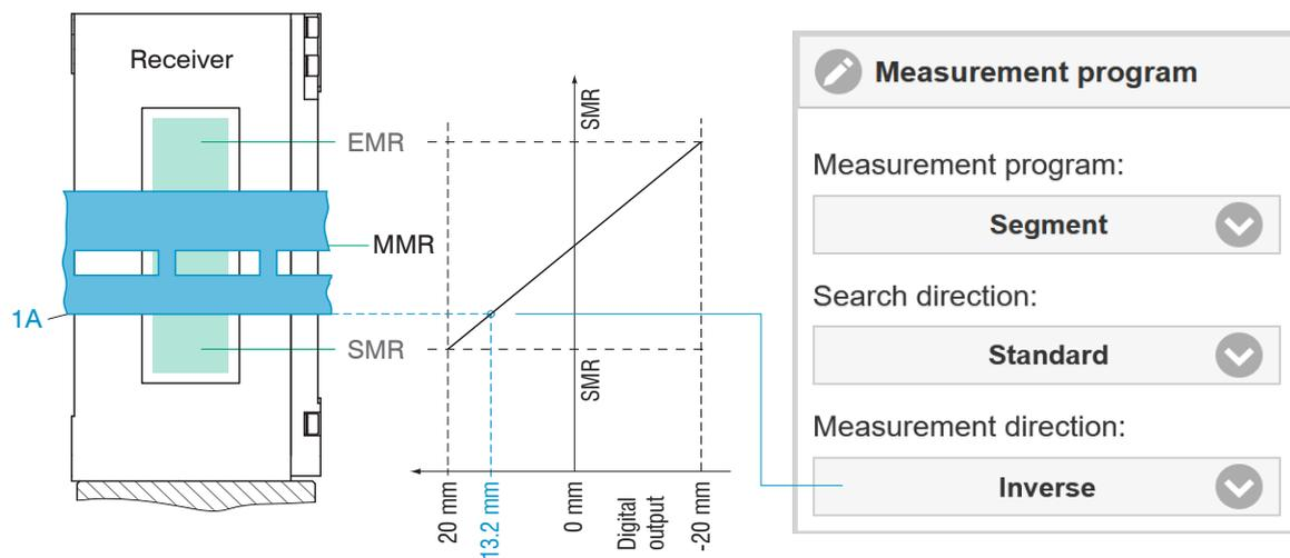
Fig. 6.8: Digital Output with Inverse Measurement Direction
