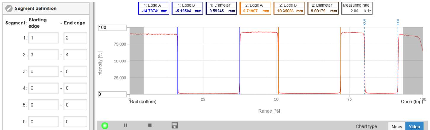
Fig. 6.9: Factory-set segment definition in the multi-segment preset
