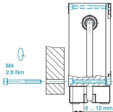
Fig. 4.6: Sensor Secured with Direct Screw Connection
