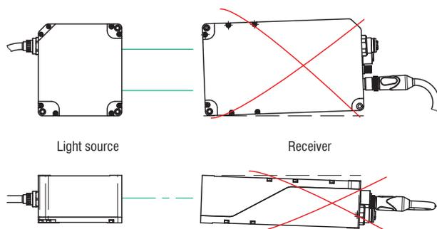
Fig. 4.7: Adjustment Errors to Avoid During Freestanding Mounting
