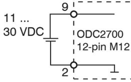
Fig. 4.5: Supply voltage connection
