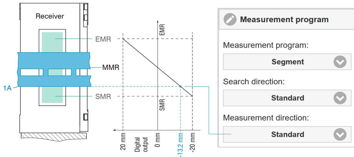
Fig. 6.7: Digital Output with Standard Measurement Direction
