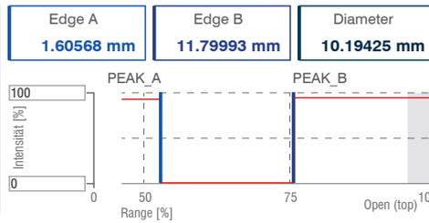
For measuring the diameter of cylindrical objects (e.g. dowel pins, bolts, bar stock, pipes, hydraulic lines). The tilt angle of the object in relation to the measurement plane is compensated for in real time by the active tilt correction.
