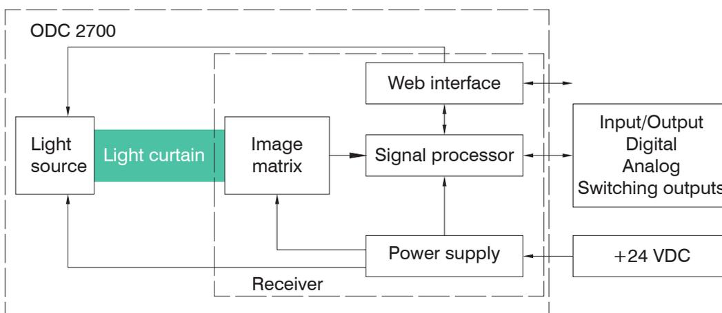
Fig. 2.5: Block Diagram of the ODC2700 Sensor
