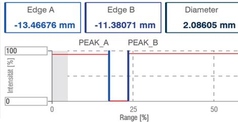
For measuring component contours on a stepped turned part. The lower edge (A), upper edge (B), center axis (C), diameter (D) and the encoder value are detected.
