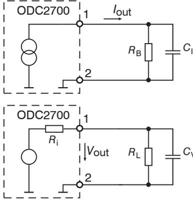
Fig. 4.6: Analog output switching
