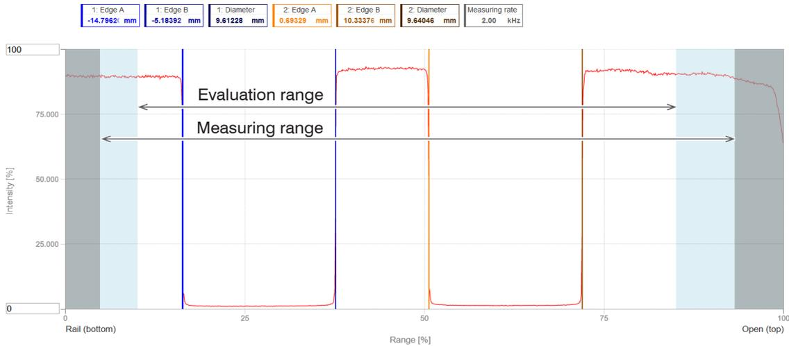
Fig. 6.11: Limiting the video signal used
