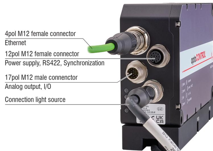
Fig. 4.12: Electrical connections of receiver
