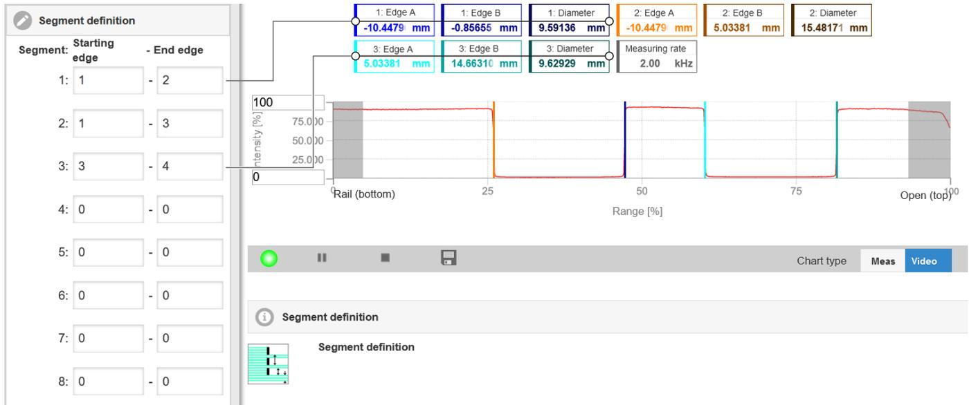
Fig. 5.4: Video Signal with Defined Segments
