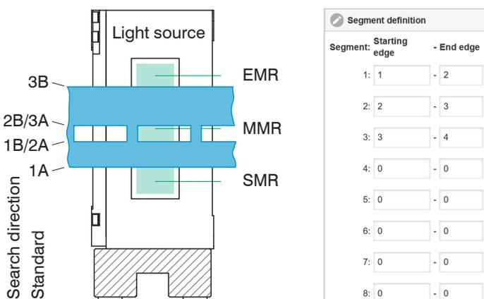
Fig. 5.4: Punching Profile with Edge Assignment (Left) and Associated Definition of Segments (Right), Viewed in Direction of Light Source
