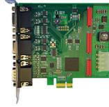
IF2008/PCIE interface card for the synchronous capture of 4 digital sensor signals or 2 encoders. In conjunction with the IF2008E, a total of 6 digital sensor signals, 2 encoders, 2 analog signals, and 8 I/O signals can be captured synchronously.
