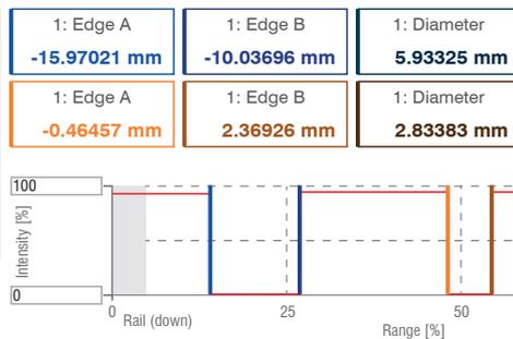
Simultaneous measurement of several objects in the beam path, e.g. strips or wires, or targeted detection of segments selected by the user. The individual definition of user and application-specific segments is possible. The Multi-segment preset enables individual assignment of the edges to each other. Detailed information is available in the Advanced settings chapter.
