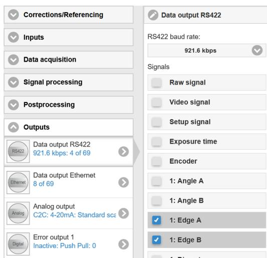
Fig. 6.22: Selection of Output Data via RS422
