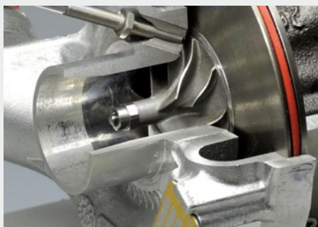
Rotational speed measurement of turbochargers
