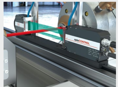
Diameter measurement of extruded products
