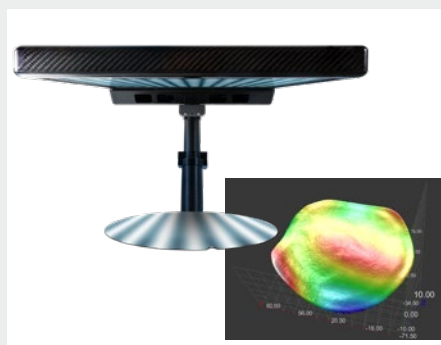
3D shape measurement of wafers
