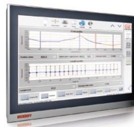
thicknessGAUGE O.IMS Sensors used: White light interferometer
