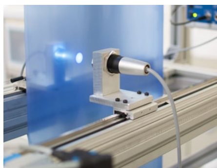
Inline color gradient measurement of transparent film and acrylic glasses
