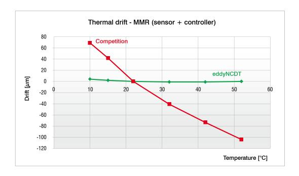
All eddyNCDT sensors and controllers are actively temperature-compensated (sensors up to max. 180 °C, controllers up to max. 50 °C). This means that the temperatures of the sensor and the controller are recorded during operation and considered in the measurement result. Consequently, you get an extremely stable measurement signal.
