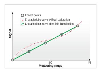
If the installation situation does not correspond to the standard installation conditions, field linearization is recommended (available with eddyNCDT 3060 and eddyNCDT 3300) This on-site calibration compensates for influences which result from the installation scenario or the target materials and shapes. Therefore, optimum measurement accuracies will always be achieved even in the case of difficult installation conditions.
